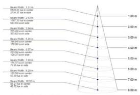
Average Beam Angle =  $66.6^{\circ}$  Max. Beam Angle =  $67.4^{\circ}$  at  $\Phi1$  =  $30^{\circ}$  –  $\Phi2$  =  $210^{\circ}$  Min. Beam Angle =  $66.0^{\circ}$  at  $\Phi1$  =  $0^{\circ}$  –  $\Phi2$  =  $180^{\circ}$
